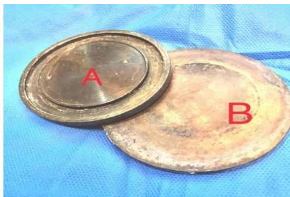
Figure 2: Finished stainless steel A: Mold, B: Cover.
