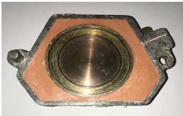
Figure 3: Stainless steel mold after investment.
