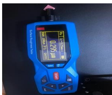
Figure 4. Contact profilometer for surface roughness measurement.
